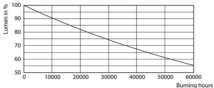
Lumen Maintenance Diagram - CorePro LED PLT HF 15W 830 4P GX24q-3
