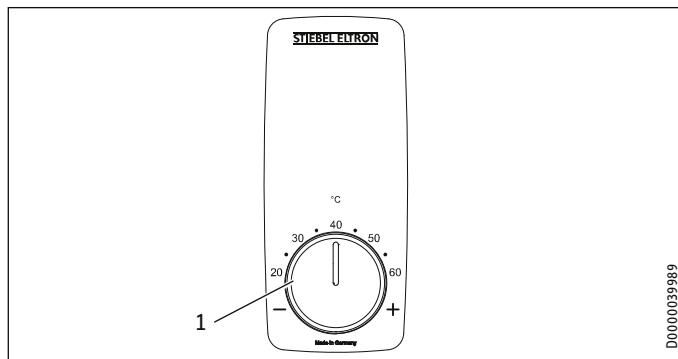
1 Temperature selector: Temperature setting range 20 °C - 60 °C
