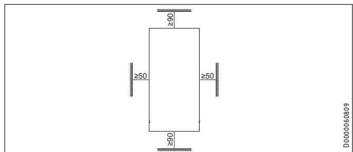
► Maintain the minimum clearances to ensure trouble-free operation of the appliance and facilitate maintenance work.
